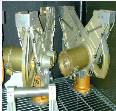
LEFT: Complex scissor/jaw docking mechanisms
