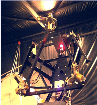
ABOVE: Air bearing sled with conceptual docking mechanisms
